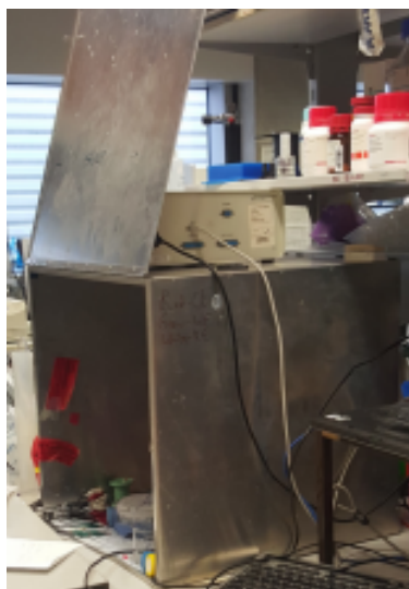
Figure 4.4: The Faraday cage used in the measurement.
