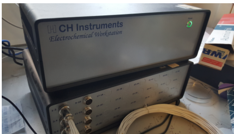
Figure 4.2: CHI760E Electrochemical Workstation by CH Instruments, Inc.
