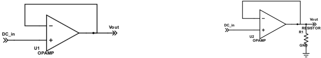
Figure 22 : Amplifier test condition 1 - no load (left), amplifier test condition 2 - with load (right)
