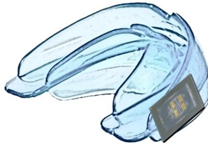
FIGURE 8.1: Envisioned SOB Fitting on retainers, with SOB covered with epoxy. The SOB is placed on the outer layer of the retainers to avoid interference with user's jaw motion.
