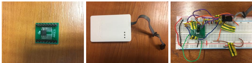
(A) ATTiny85 on SOIC-DIP (B) ATMEL ICE Programmer (C) Breadboard Connections
