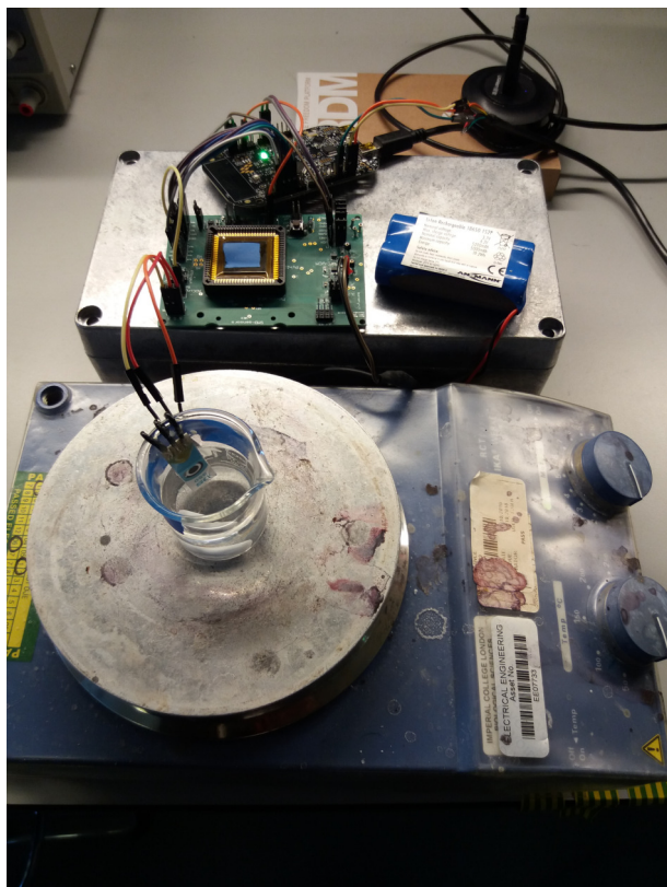
Figure 3.17: Prototype setup for electrochemical measurements
